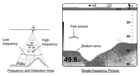
Frequency and detection area, sample single picture (low frequency)
